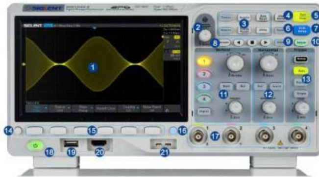
Figure 9 4-channel Scope Front Panel Overview
